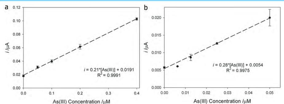
**Figure 5.** a) Calibration curve for As(III) at high concentration range (i.e. 0.05  $\mu$ M to 0.4  $\mu$ M or 3.75 ppb to 30 ppb) determined with the data obtained from Figure 4. b) Calibration curve for As(III) at low concentration range (i.e. 0.0125  $\mu$ M to 0.05  $\mu$ M or 0.94 ppb to 3.75 ppb) determined in a separated experiment (data not shown). LOD = 0.0105  $\mu$ M or 0.8 ppb. The error bars represent the calculated standard deviation from triplicates.
