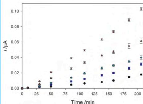
**Figure 4.** Amperometry detection of PAP as a function of time for different As(III) concentrations: 0  $\mu$ M (0 ppb, Filled Black Circles), 0.05  $\mu$ M (3.75 ppb, Filled Blue Squares), 0.1  $\mu$ M (7.5 ppb, Filled Cyan Diamonds), 0.2  $\mu$ M (15 ppb, Filled Brown Triangles), 0.4  $\mu$ M (30 ppb, Filled Red Stars). The error bars represent the calculated standard deviation from triplicates. The recorded response is proportional to the As(III) concentration.
