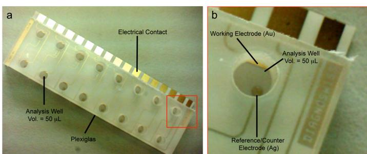
**Figure 3.** a) Optical photograph of the microchip employed for the stop flow measurements of As(III). The microchip contains 16 independent electrochemical sensors each one consisting of a two-electrode setup (working electrode = Au, counter/reference electrode = Ag) and a well made in Plexiglas (see Figure 3b).
