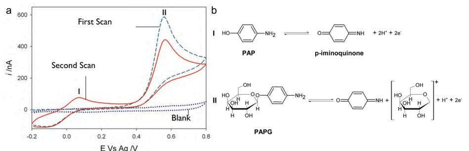
**Figure 2.** Electrochemical monitoring of PAP. a) Cyclic voltammetry of PAPG 1 mM in PBS 1x (pH = 7), first scan (cyan dashed line), second scan (red continuous line) and supporting electrolyte PBS 1x (blue dotted line). Scan rate = 20 mV/s. b) Electrochemical reactions taking place at I (i.e. PAP oxidation) and II (i.e. PAPG oxidation). By working at a constant potential of 0.05 V Vs Ag, the production of PAP can be monitored electrochemically.
