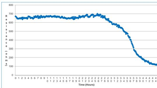
Fig6: Shows continuous TEER measurements taken over a period of 44 hours on fully differentiated C2Bbe1 cells and a drop in TEER in response to a toxicant
