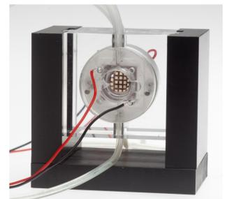
Fig4: The system is integrated into a fluidics device and clamped together to ensure water tightness
