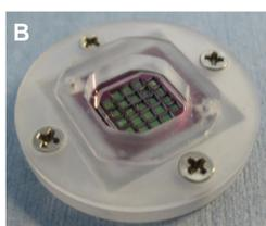
Fig3: **A** Silicon Nitride permeable insert with 23 silicon nitride pads and integrated platinum electrodes **B** Shows the custom holder for the membrane
