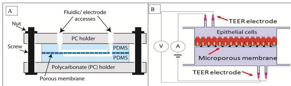
Figure 2. Cross-sectional schematic representation of the clamping holder for the microfluidic chip (A) with indication of the 4 TEER electrodes (B).
