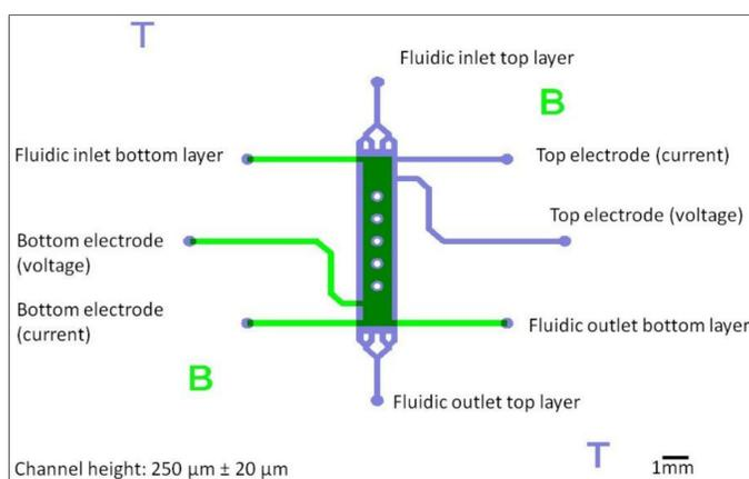
Figure 1: Schematic representation of the two-layer mask design (layers B(bottom) and T(top)) of a microfluidic chip for TEER measurements. To avoid membrane collapse, five PDMS posts are used in the center of the chamber as membrane support.
