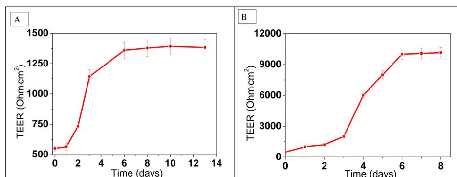
Figure 5. Time dependence of the TEER of a Caco2 cell monolayer cultured in a Transwell device (A) and on the microfluidic chip (B).
