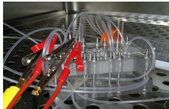
Figure 3. Photograph of a clamped microfluidic chip with connectors for the TEER measurements.
