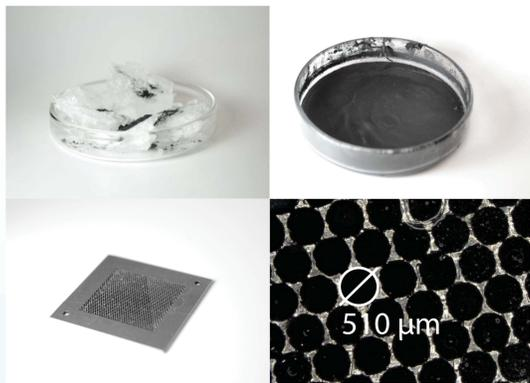
Paraffin wax is mixed with carbon black (a) and filled into the honeycomb hole array (b) in order to create the actuator. PDMS is spincoated on top to create a flexible membrane and the actuator is sealed on the back with a glass slide (c). d) Top view onto the steel actuator (bright) filled with paraffin wax/carbon black
